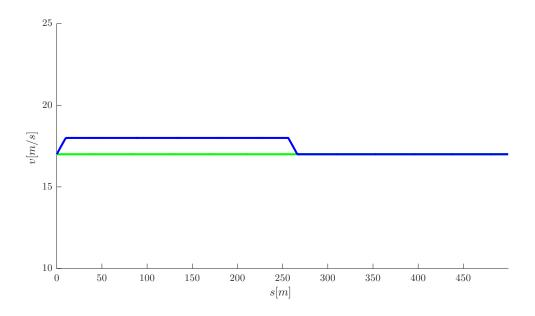
Figure 7.13: Comparison of ecoAD overtaking and state-of-the-art optimal overtaking  $(LQ \ deviation)$ .
