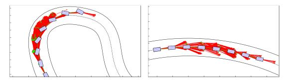
Figure 7.6: Graphical representation of the trajectories exploration in U-turn (left) and wide turn (right).
