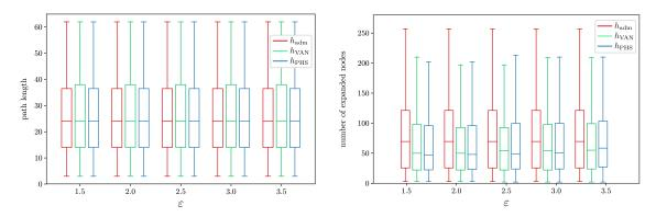
Figure 7.20: Path length (left) and number of explored nodes (right) for  $h_{\rm adm}$ ,  $h_{\rm VAN}$  and  $h_{\rm PHS}$  heuristic based on  $\varepsilon$  value.
