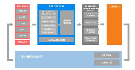
Figure 2.3: Autonomous Vehicle architecture.
