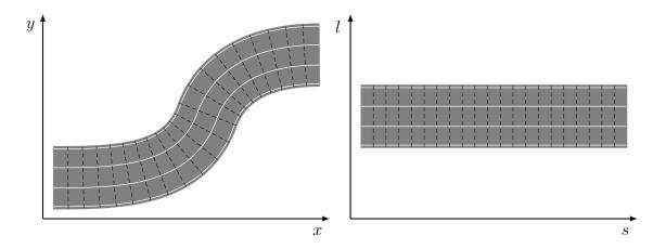
Figure 5.5: Curvilinear road representation (Cartesian and Frenet-frame).
