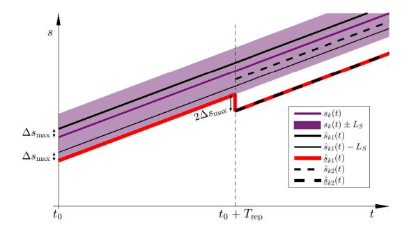
Figure 6.14: Predicting movement of other vehicle - linearization.
