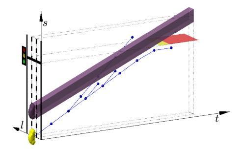
Figure 5.11: Automated Driving behavior and motion planning problem.
