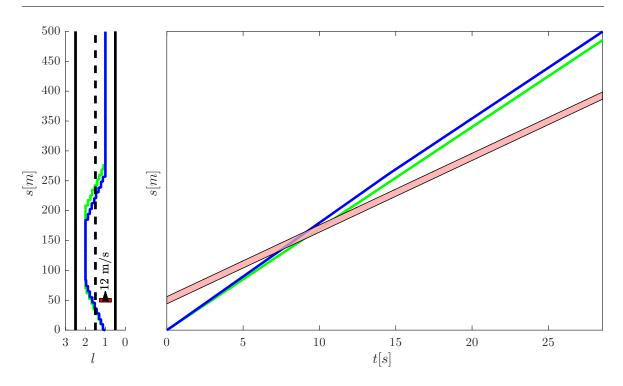
Figure 7.12: Comparison of ecoAD overtaking and state-of-the-art optimal overtaking  $(LQ\ deviation)$ .
