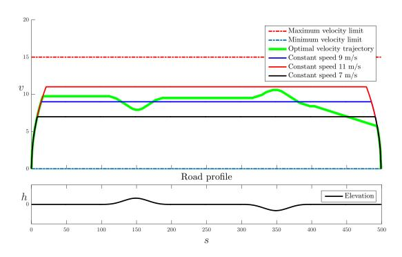
Figure 7.10: Benchmarking ecoCC and constant speed driving.
