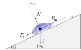
Figure 5.1: Vehicle on a slope, the force balance.
