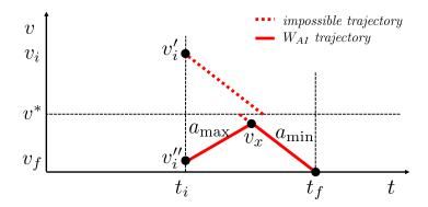
Figure 6.9: Special cases of velocity trajectories for  $W_{AI}$  computation.
