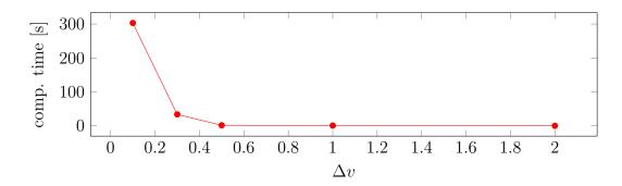
Figure 7.17: Influence of the  $\Delta v$  step ( $\Delta s = 10 \text{ m}$ ,  $\Delta t = 1 \text{ s}$ ,  $T_{\text{hor}} = 20 \text{ s}$ ) on computation time of SBOMP in Automated Driving.
