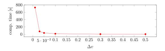
Figure 7.16: Influence of the  $\Delta v$  step ( $\Delta s = 5$  m,  $S_{hor} = 18000$  m) on computation time Dynamic Programming for Energy-efficient Driving.
