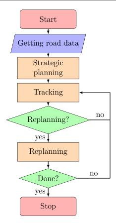
Figure 6.10: Optimal motion planner flowchart.
