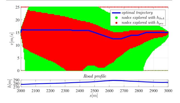
Figure 7.11: Space searched by using different heuristics.
