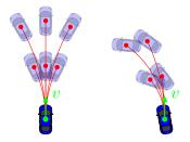
Figure 6.17: Motion primitives for performance driving using semi-linearized bicycle model (left) and ESM (right).
