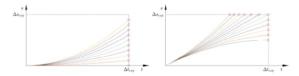
Figure 6.11: Expanding parent node n to different child nodes n' by piecewise constant acceleration, from initial velocity v = 0 (left),  $0 < v < v_{\text{max}}$  (right).
