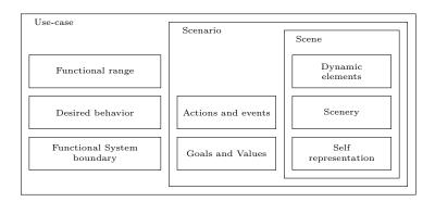
Figure 4.1: Scene, Scenario and Use-Case definitions based on [221].
