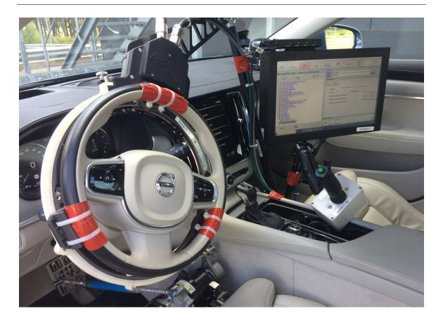
Figure 8.9: Steering robot used for executing driving trajectories.
