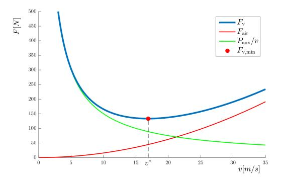
**Figure 6.6:** Velocity-dependent virtual force  $F_{\rm v}$ , generated by combined air drag resistance and auxiliary power.
