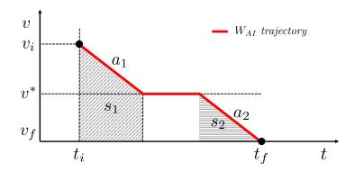
Figure 6.8: Velocity trajectory for  $W_{AI}$  computation.
