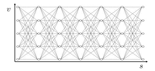
Figure 6.2: Search space for Energy-efficient Driving problem constructed as a graph.
