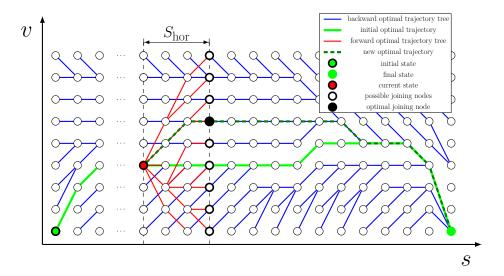
Figure 6.15: Forward Dynamic Programming-based replanning.
