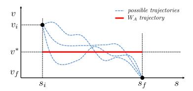
Figure 6.7: Some of possible trajectories for driving from initial to final state, and lower bound trajectory for  $W_A$  computation.
