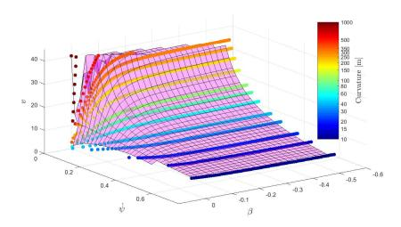
Figure 5.4: Equilibrium points sets  $S_{ss}$  (and linear interpolation) in the  $v, \beta, \dot{\psi}$  space for counter-clockwise cornering maneuvers with different curvature radii  $R_c$ .
